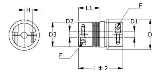
D = 109Nom. torque NM (Tkn) = 200NM overload torque range 2 D1 = 38Position engagement = C = Synchronous
